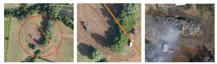
**InstiMaps Sensors.** Airborne sensors include high resolution visible and thermal infrared cameras. When flown at 1500' AGL, the visible camera provides 3" resolution imagery of a 1,250' wide corridor over asset centerline. The infrared camera spots and reports fires within 250' of the corridor centerline.
